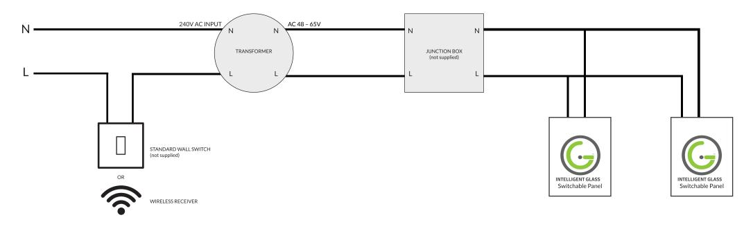
**Receiver Wiring Diagram**
